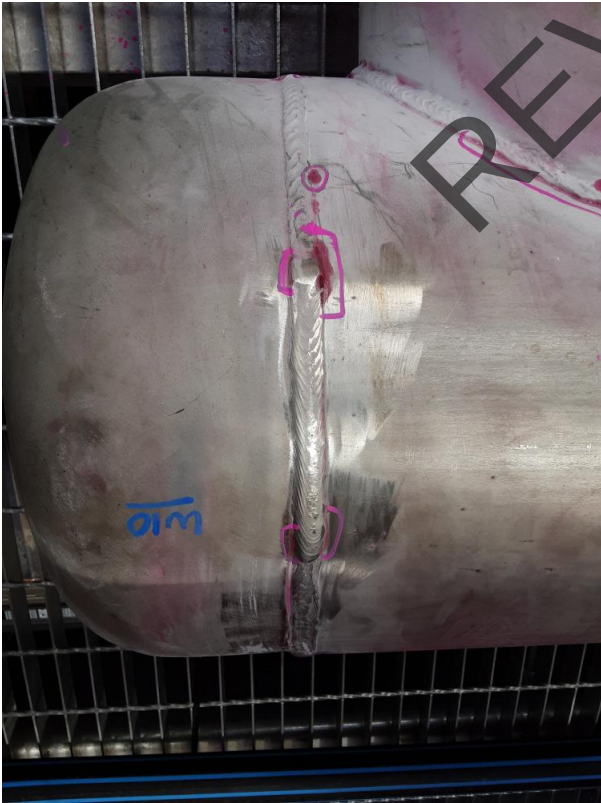
Image 11 of 13 - BTM SP3 W10: Intermittent Lack of fusion entire weld length up to 100mm
